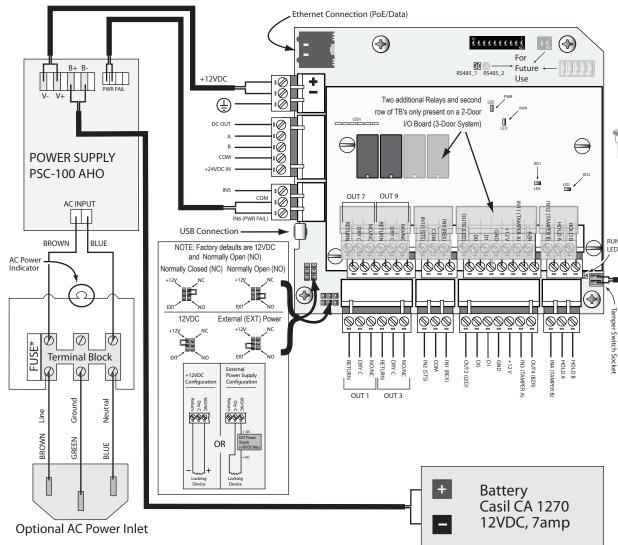
All field wiring except for the battery backup / charger wiring is Class 2 Power Limited.
